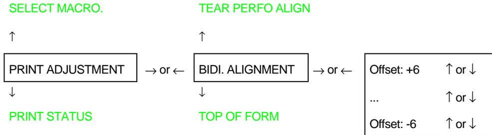
This function adjusts the bidirectional printing in a range between - 6 and +6. When the previous value is changed, the printer prints two ‘|’ lines to control the final output.
