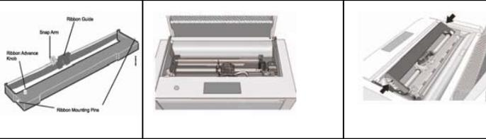
The ribbon must be between the print head nozzle and the mask.
