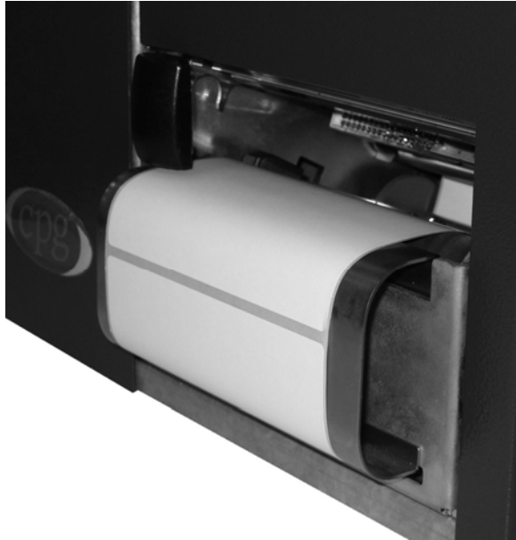
Fig. 22 – Detail of the paper path in the rewinder guide
